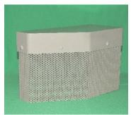
while being durable enough to withstand deliberate destruction. The entire body is formed from 12 gauge perf with 1/8 dia holes on 3/16 staggered centers, while all end caps, splice plates, corner panels, closure boxes, etc are 14 gauge solid. Uses for our crownline covers include all types of institutional, public housing, commercial and industrial applications
