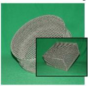
body is formed from 16 gauge perforated steel (3/16 dia perforations on 1/4 staggered centers) giving it a 51% open area which does not interfere with detector
